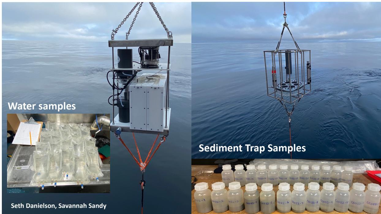
Figure 2.15.5. Water samplers (left photo) and sediment trap (right photo) at the CEO mooring site.
