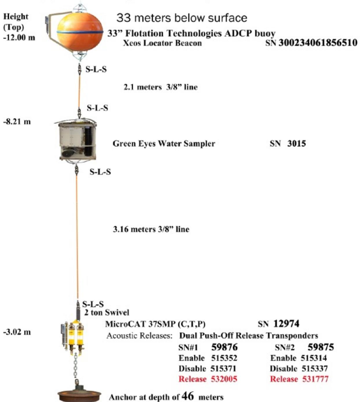
Figure 2.15.1 Mooring CEO1-23 as deployed during SKQ22-12S.
