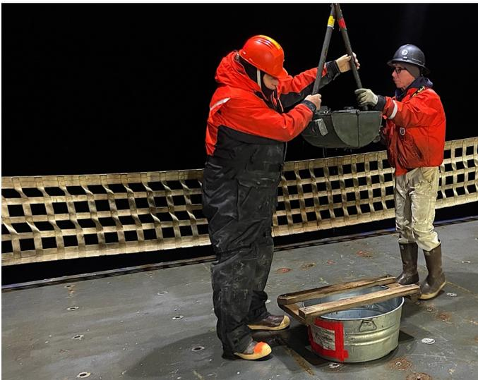
**Figure 2.9.1.** Use of van Veen grab for sampling sediments.
