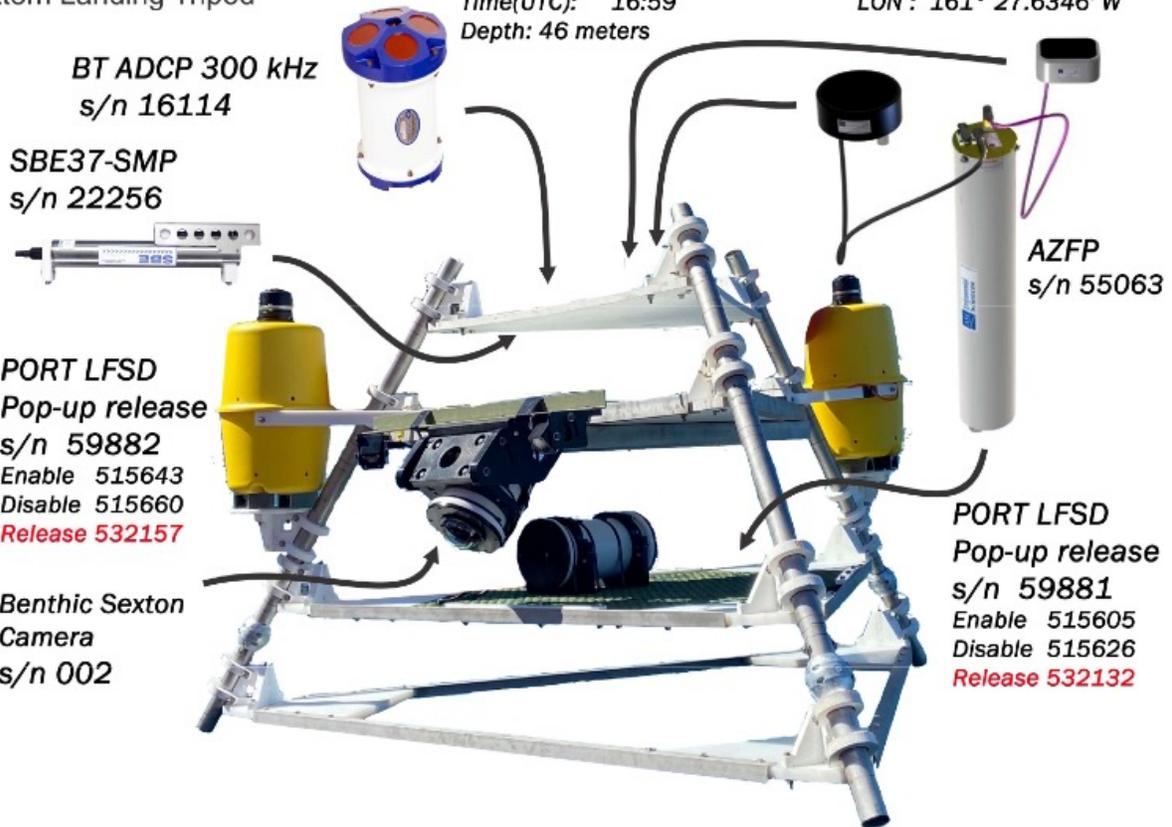
Figure 2.15.3 CEO3-23 Tripod mooring as deployed during SKQ22-12S.
